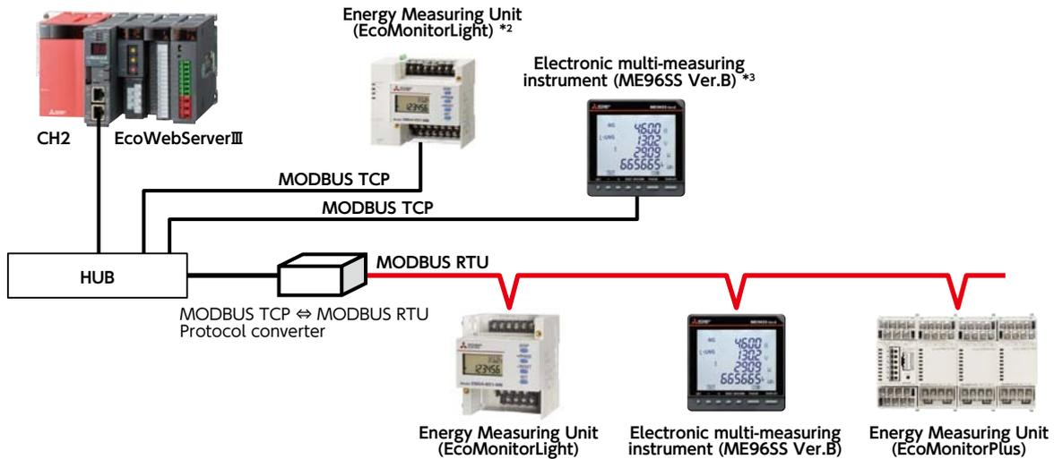
\*1 MODBUS TCP ⇔ RTU converter is required for MODBUS RTU communication.
