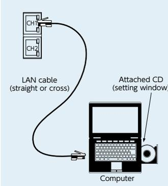
When connecting the PLC (CH2)
