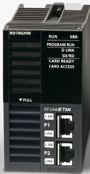
CC-Link IE TSN-compatible motion module
