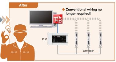
Positioning data is written from the Positioning Communication Protocol Support Tool to the controller, thereby eliminating wiring between computers and controllers.
