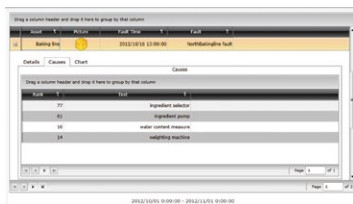
When an error occurs, possible causes are ranked according to the conditions surrounding the error
